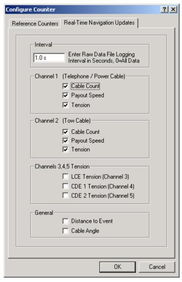
This tab enables/disables certain data from this device to be passed to the vehicle. Unlike the Reference Counters tab, data from the Real-Time Navigation
