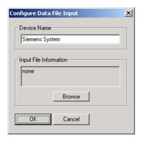
The Siemens System writes cable data to an ASCII file. WinFrog reads the cable data from this file over the network. Click the Browse button to select the appropriate data file.
