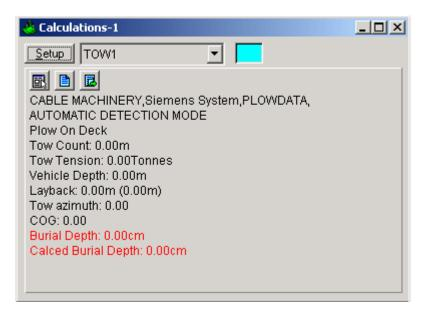
From this window you can monitor some of the input data, as well as the layback calculation. This calculation window also provides a shortcut to the Configure Plow dialog box by clicking on the button.
