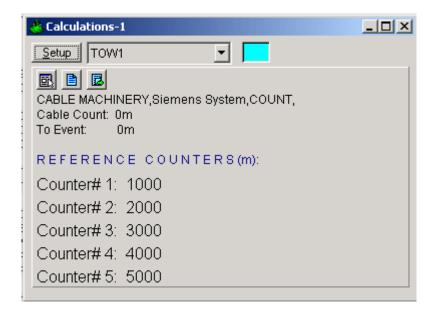
Once the Calculations window has been opened and configured, the five reference counters can be modified using the Reference Counters tab of the Configure Counter dialog. (Note: the Configure Counter dialog can be directly accessed from the Calculations window by clicking the licon in the Calculations window.)
